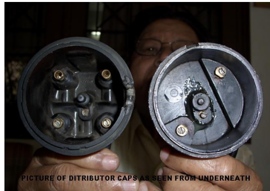
Picture of distributor caps as seen from underneath
