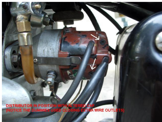
Distributor in position with altered cap. (Notice the dummies used closing extra wire outlets)
