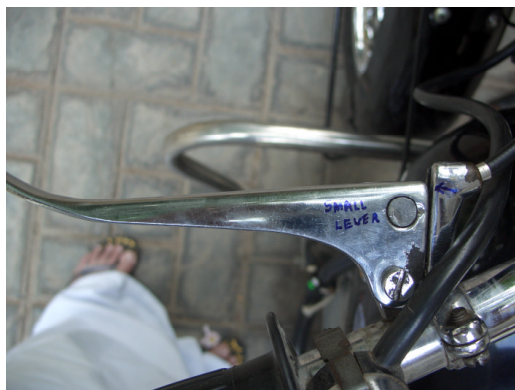
Incorrect lever fitted originally when the machine was received.
