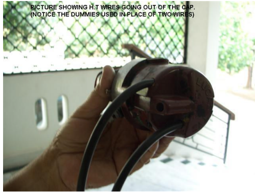
Notice the dummies used in place of two wires
